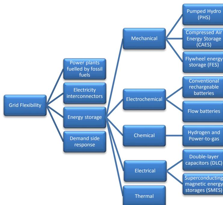
Figure 1 Technological solutions for grid flexibility.
