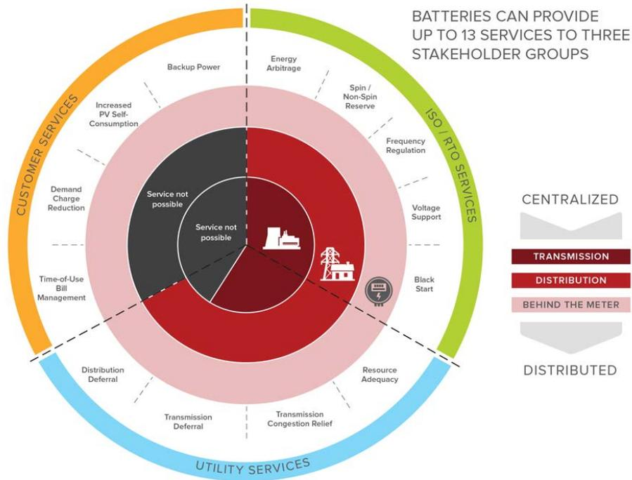
Figure 5. Different services by batteries (RMI, 2015)
